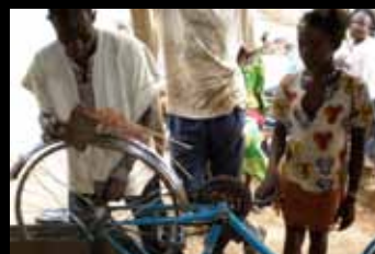
Mahangurina [pearl millet] thresher , prototype. Michelle Marincel, George Yaw Obeng, Thalia Konaris, Francisco Rodriguez, Brian Rasnow and mentor Donna Cohn. Designed United States and Ghana, 2008–9; deployed Mali, 2009. Scrap bicycle, conduit and metal, spring steel, cardboard. Photo: F. S. Rodriguez-Sanchez
